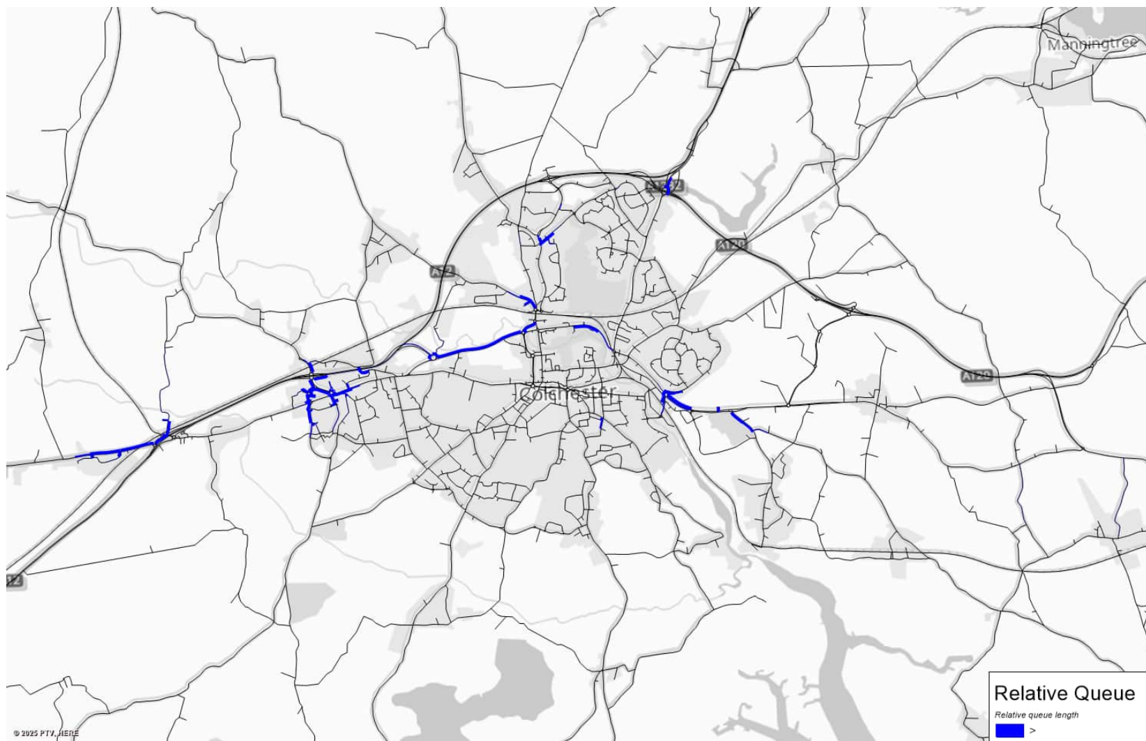
Figure E.12: Relative queue – Scenario 3 without A12 widening and delayed A1331 completion – AM
