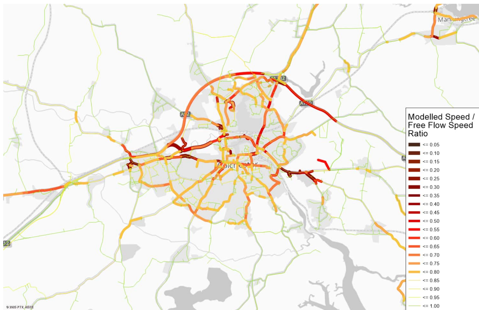
Figure G.4: Speed ratio – Scenario 0 with A12 widening and delayed A331 completion – AM
