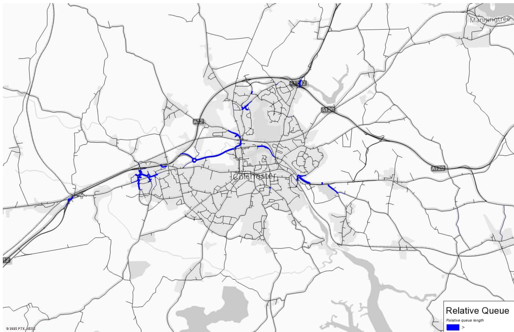
Figure G.12: Relative queue – Scenario 3 with A12 widening and delayed A1331 completion – AM
