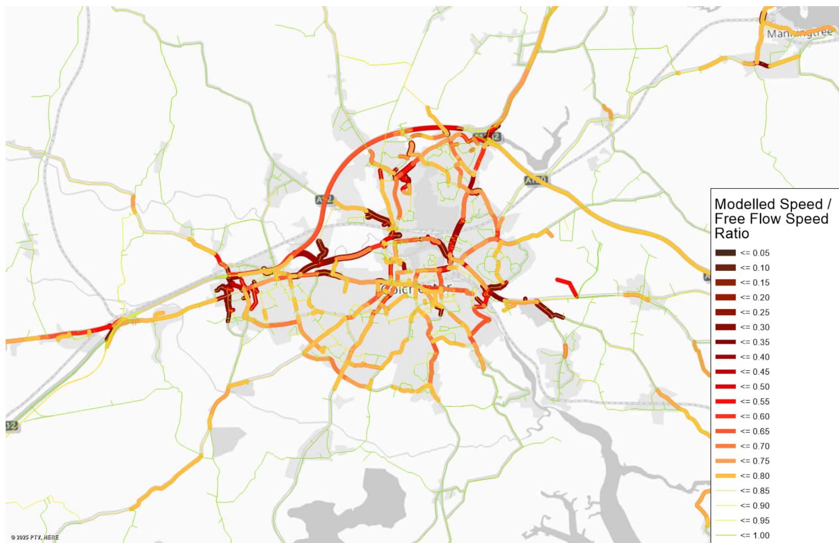
Figure G.6: Speed ratio – Scenario 2 with A12 widening and delayed A331 completion – AM
