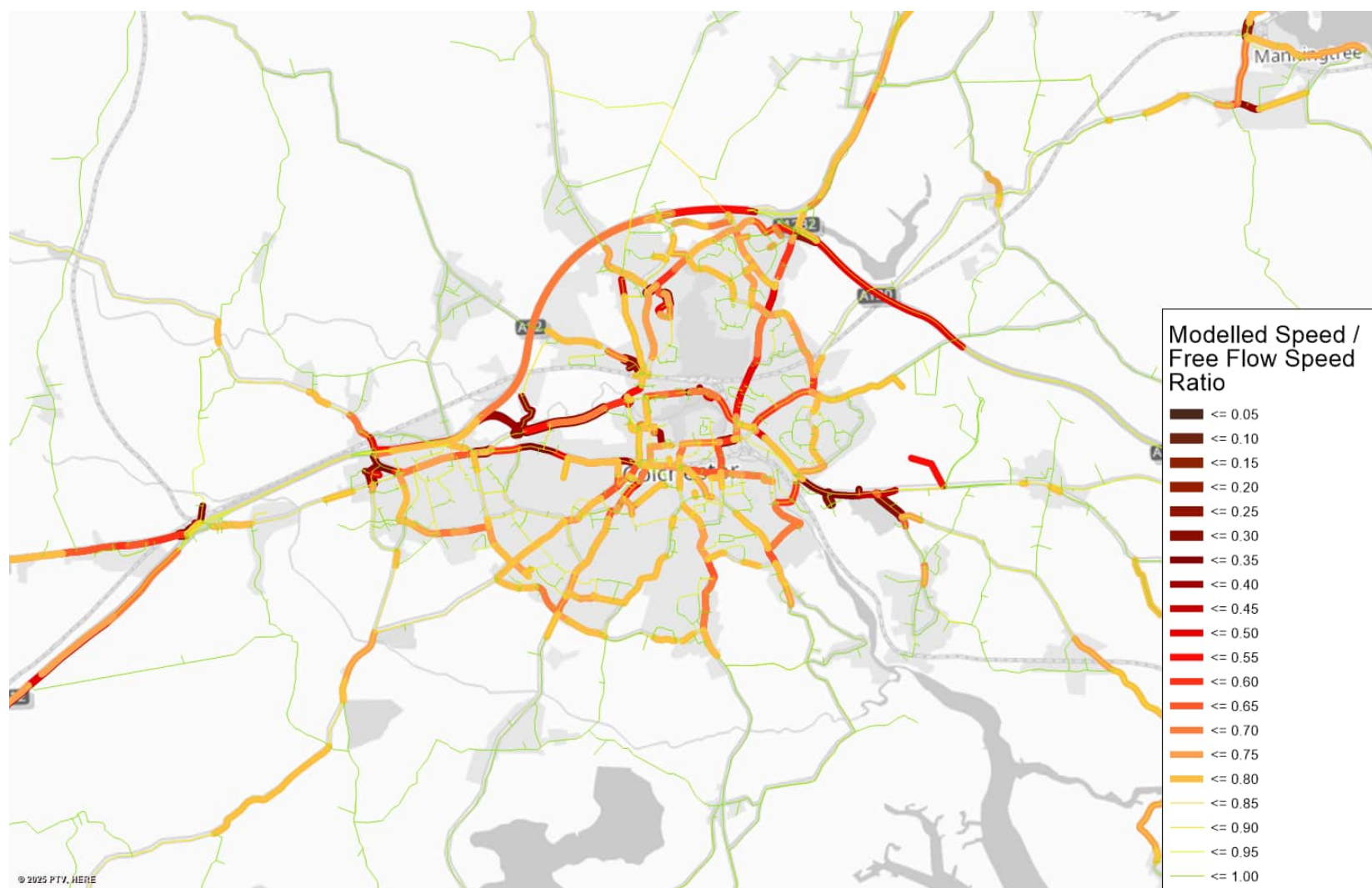
Figure E.4: Speed ratio – Scenario 0 without A12 widening and delayed A331 completion – AM
