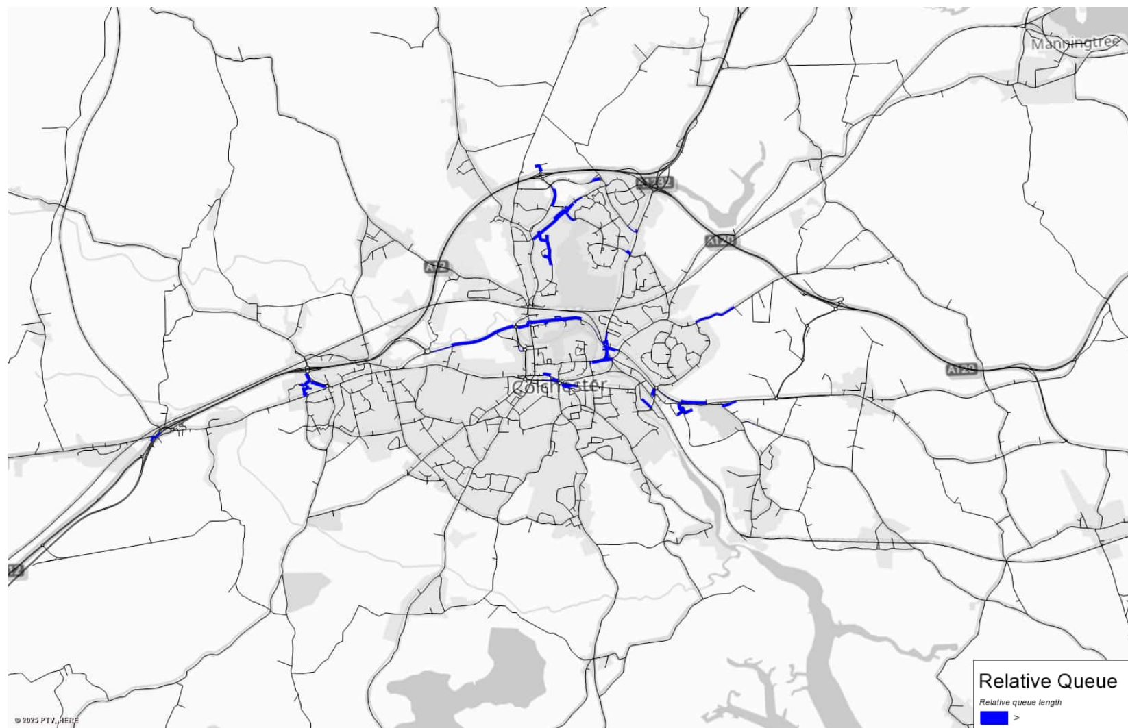
Figure F.24: Relative queue – Scenario 2 with A12 widening and A1331 completion – PM
