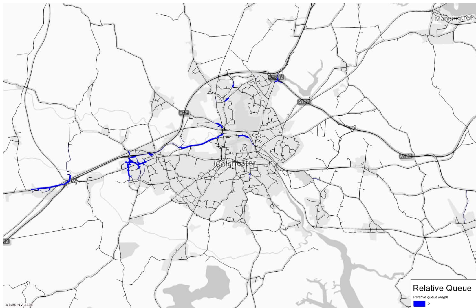
Figure D.12: Relative queue – Scenario 3 without A12 widening and with A1331 completion – AM
