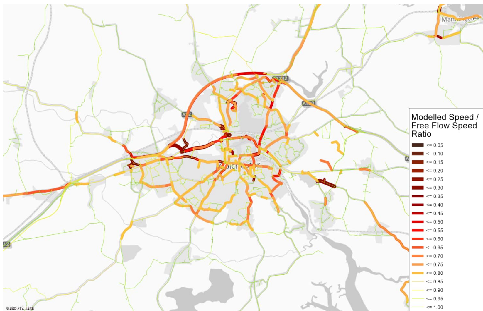
Figure F.5: Speed ratio – Scenario 1 with A12 widening and A331 completion – AM
