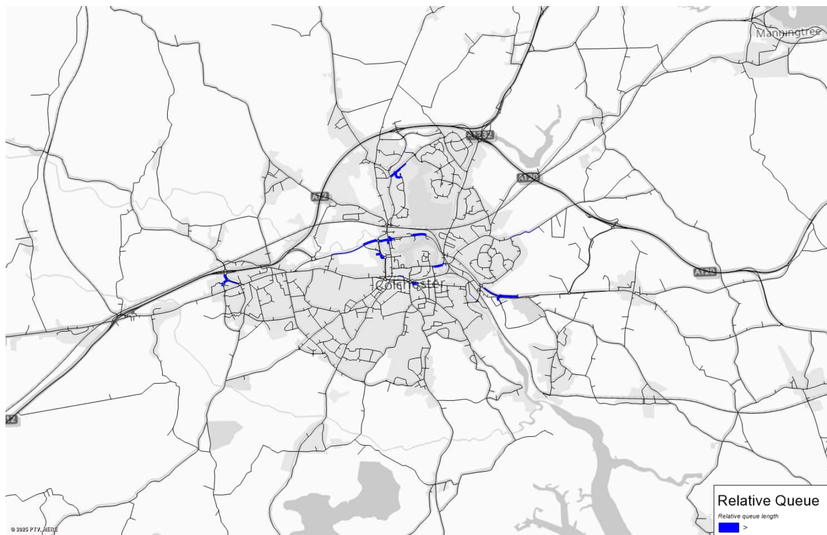
Figure E.23: Relative queue – Scenario 1 without A12 widening and delayed A1331 completion – PM
