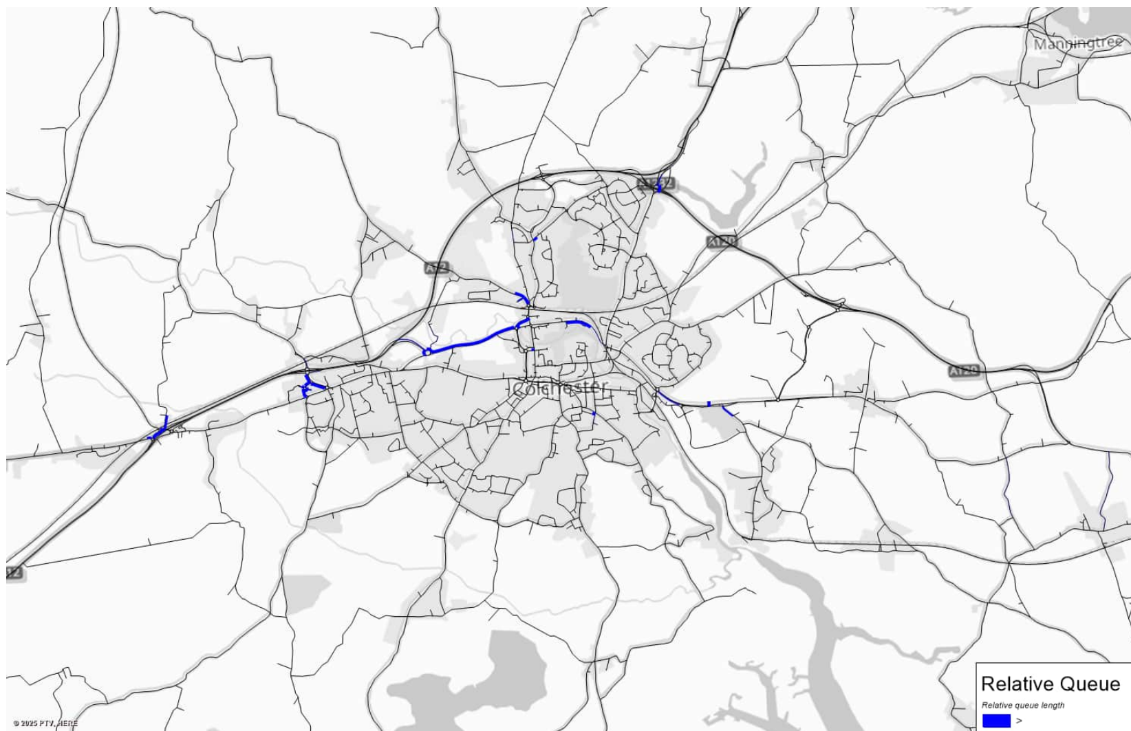
Figure E.10: Relative queue – Scenario 1 without A12 widening and delayed A1331 completion – AM
