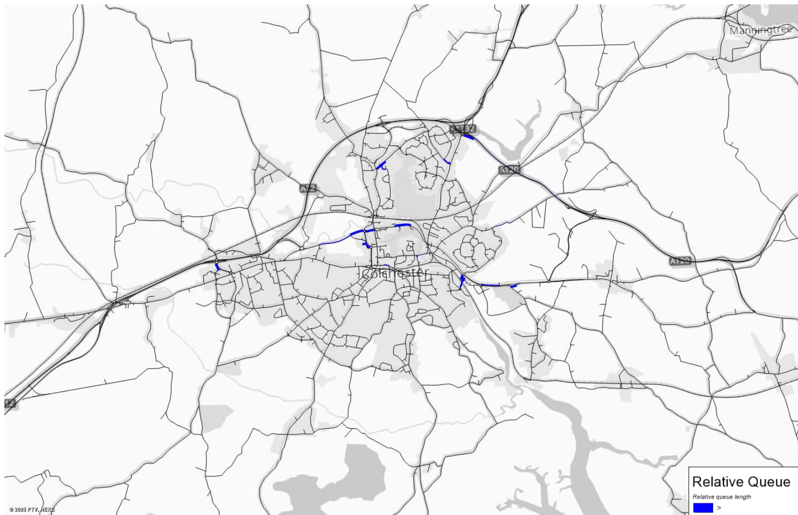
Figure F.22: Relative queue – Scenario 0 with A12 widening and A1331 completion – PM
