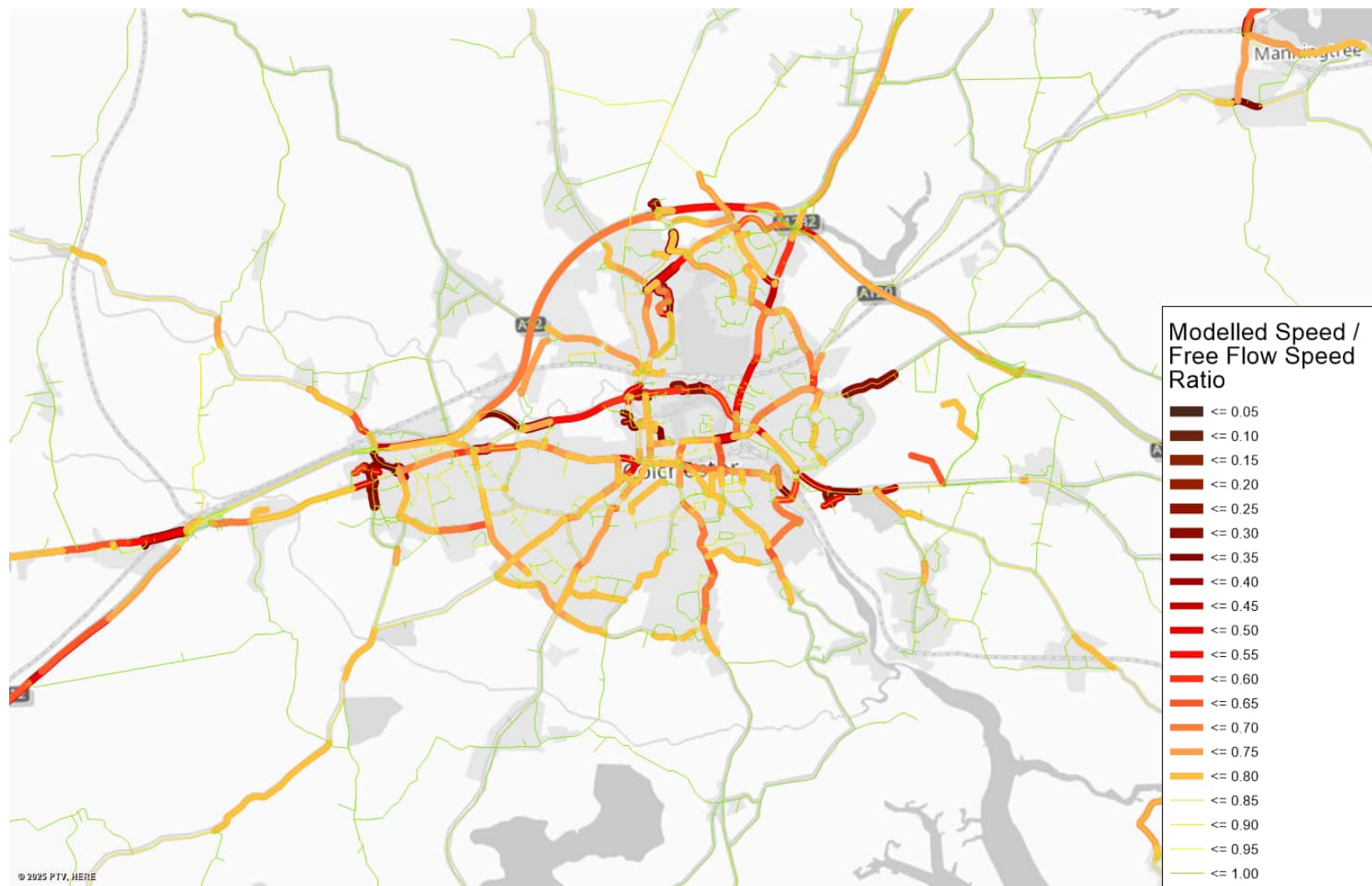
Figure D.20: Speed ratio – Scenario 3 without A12 widening and with A331 completion – PM
