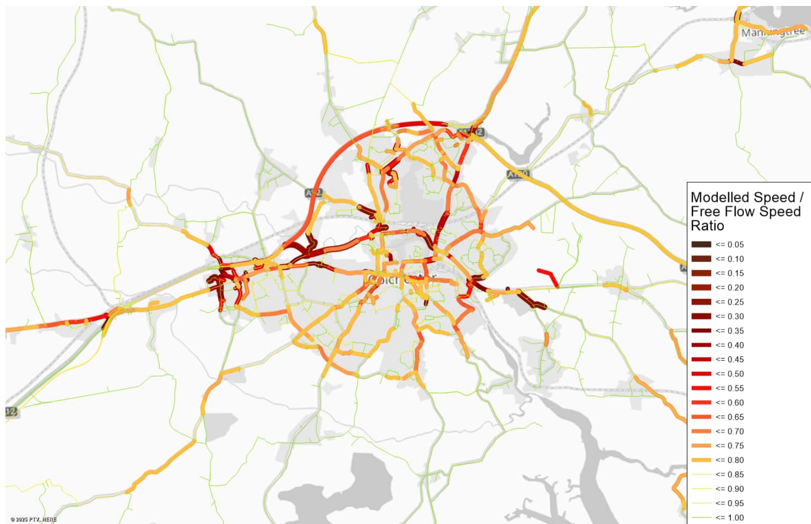
Figure G.7: Speed ratio – Scenario 3 with A12 widening and delayed A331 completion – AM
