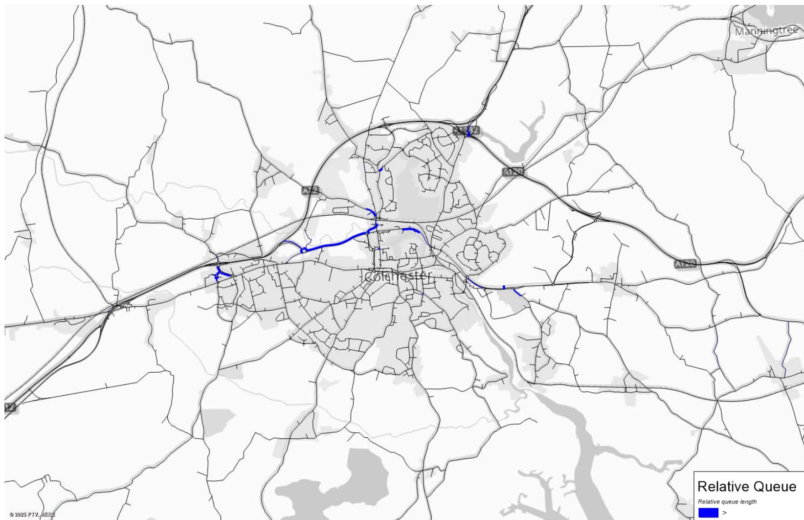
Figure G.10: Relative queue – Scenario 1 with A12 widening and delayed A1331 completion – AM
