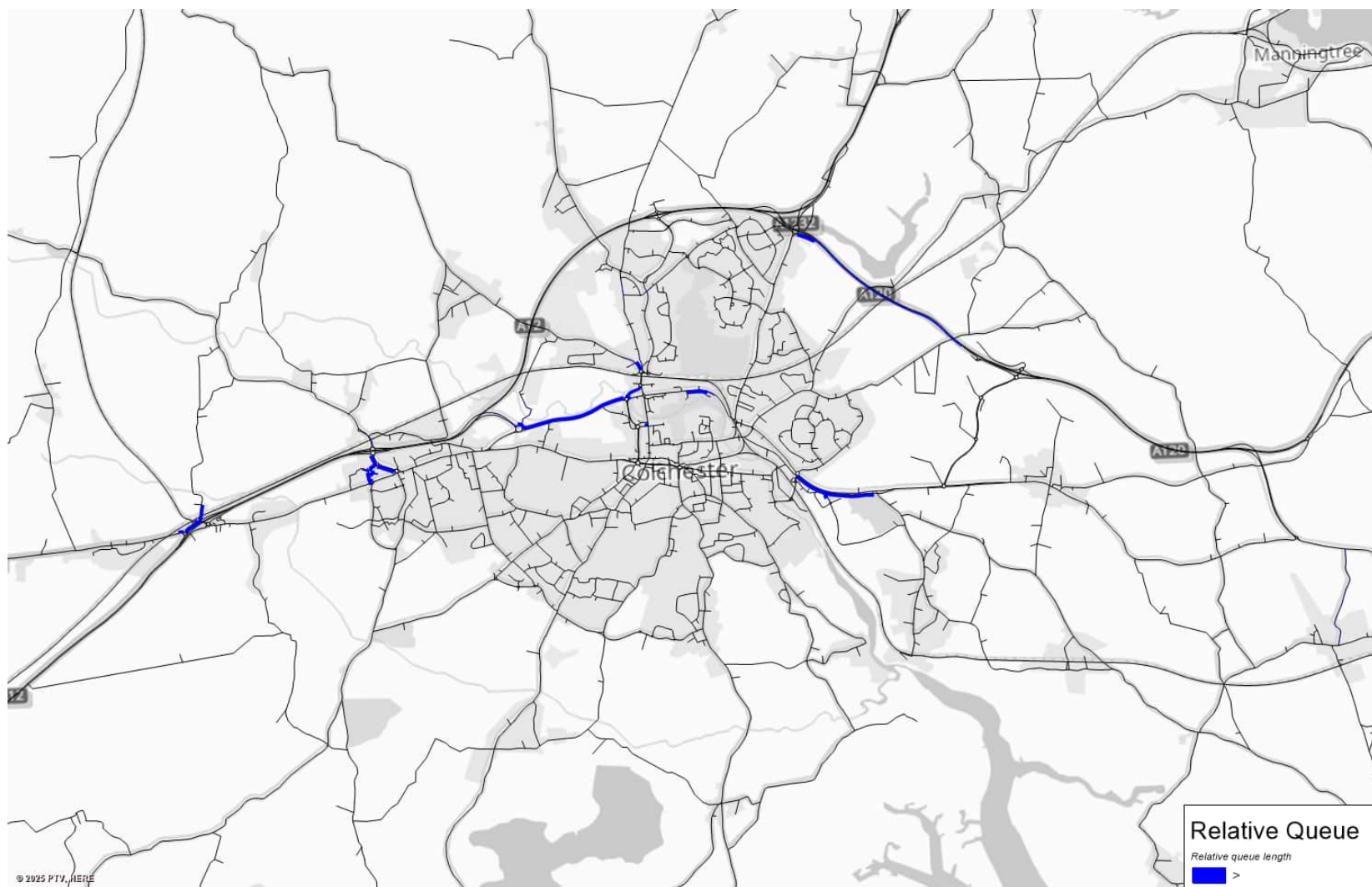
Figure D.9: Relative queue – Scenario 0 without A12 widening and with A1331 completion – AM
